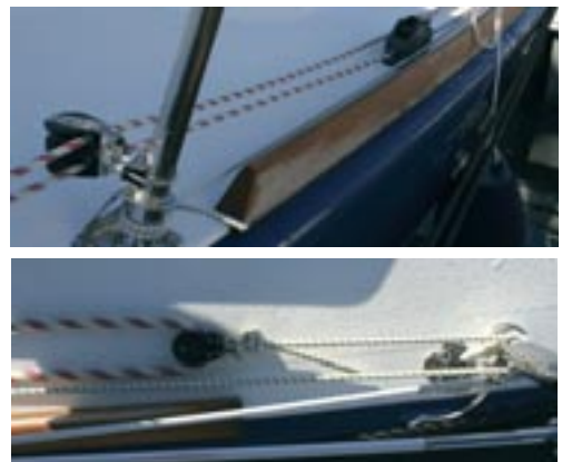
Continuous furling line installed with a jammer
